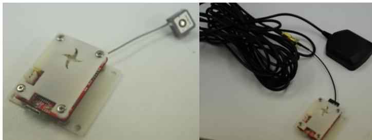
GPS antenna should be towards the sky. Position will not output if antenna doesn't see the GPS satellites.
