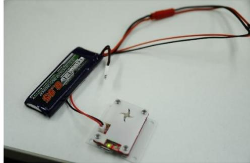
Never use a LiPo battery that show any damage or disfigurement of any kind. Swelling is a sign of internal damage. Disposal of LiPo batteries requires special care. LiPo battery for NinjaScan is 1S (3.7V).
