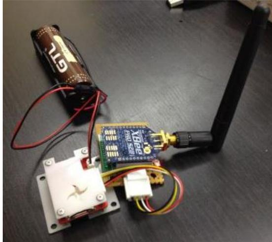
For example in the case of Xbee, you may connect as follows. In another case of another radio module, you may connect the UART pins of the logger to the pins of the input and output of the radio module.
